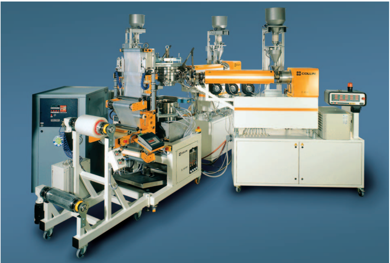
3-layer quenching line for the production of infusion bags
