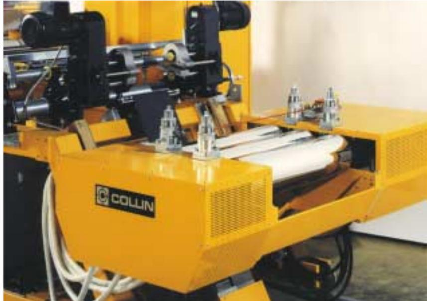
*Edge cutting with motor-driven circular blades.*
