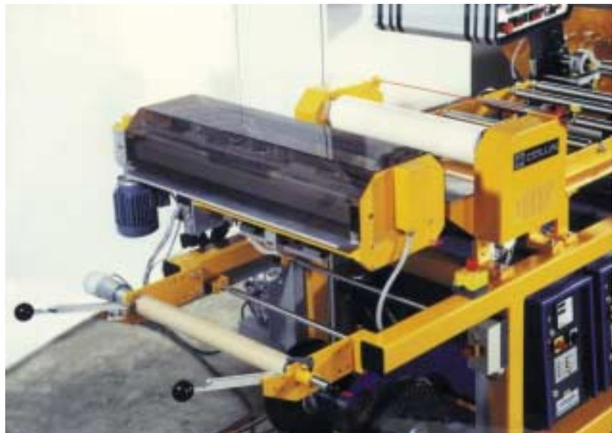
*Take off with winder for film or traversing saw for cutting sheet.*
