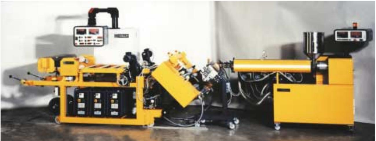
Laboratory sheet line with extruder, 45 mm diam. x 25 D, slot die 450 mm on a mobile frame, roll unit in 45° position, motor-driven edge cutting unit, take-off rolls, traversing saw, film winder, edge-strip winder and integrated hot water temperature control units.
