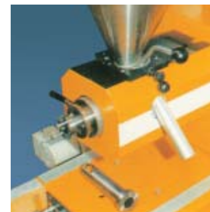
Divided barrel with interchangeable grooved bush
