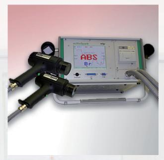
With the mIRoSpark it is possible to analyze independently of surface structure, contamination and colours the following relevant plastics, mixtures and additives:
