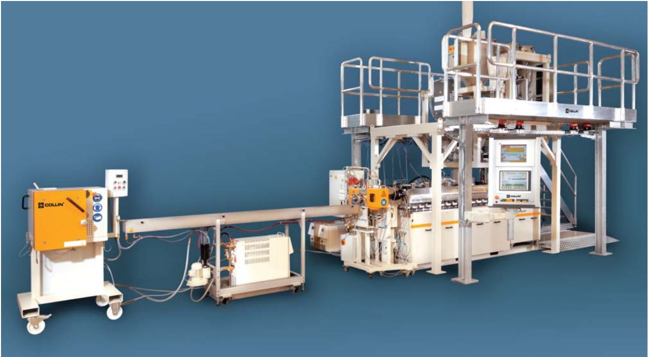
ZK 35 equipped with 4 gravimetric dosing stations for solid materials and 3 tempered liquid gravimetric stations
