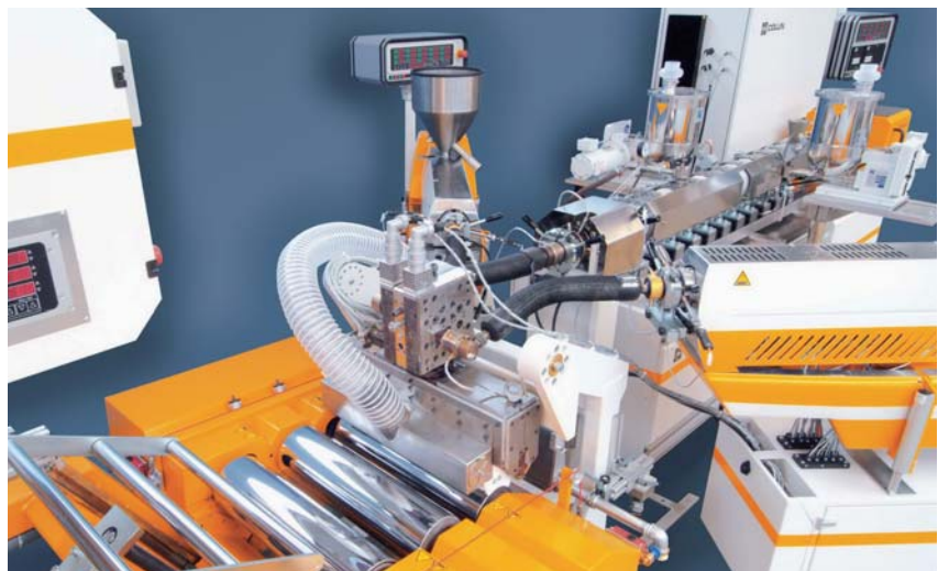
5 Layer coextrusion flat film line with direct extrusion of the central layer
