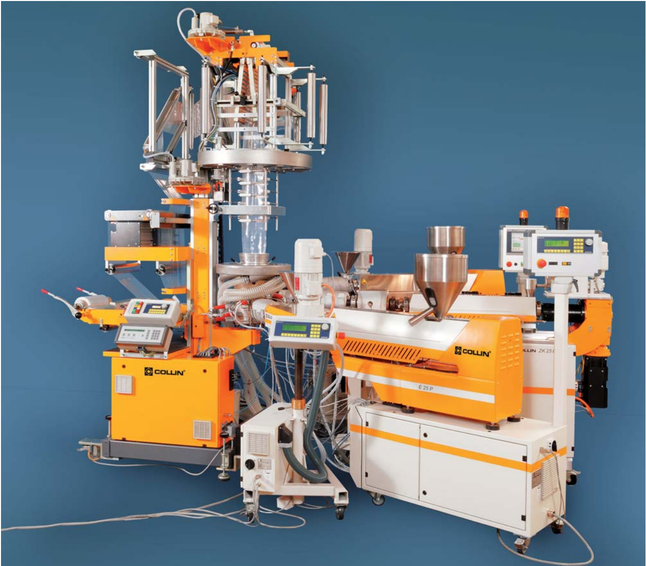
5 Layer coextrusion blown film line with direct extrusion of the central layer
