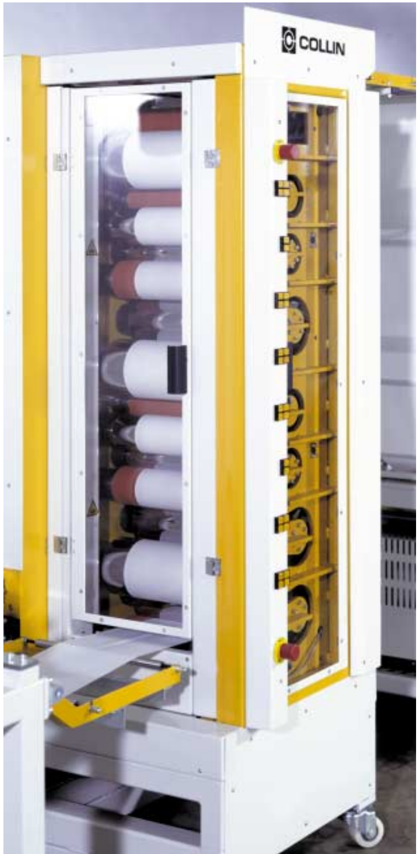
The Stretching Unit with closed safety-doors. The easy access from all sides enables less downtime for start-up and cleaning.
