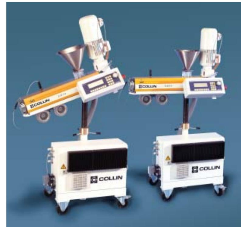
The extruder is a special design with separate electric cabinet. The extruder is mounted to allow for both rotation and height adjustment. The design has a very small footprint and is therefore the ideal machine to build up 3-, 5- or 7-layer co-extrusion lines. This type of extruder can also be combined with the bigger Extruders Type E or P of the series of pilot machines.
