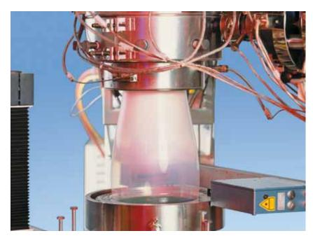
provides accurate thickness distribution. The maximum lay-flat width is 530 mm.
