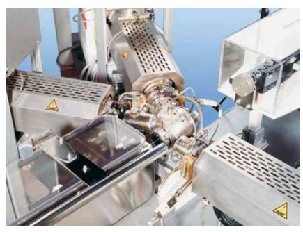
The materials used are polyolefins and polyurethanes, flexible PVC and polyamides. The line covers the diameter range between 0.5 mm and 5 mm at a maximum line speed of 100 m/min.
